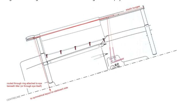
Note: routing of lines is allowed to be both internal (with new apertures cut in the racks for 'through deck' type blocks) and external. If routing is external, then utmost care must be taken to ensure that lines do not create a trip or trap hazard for the crew.
